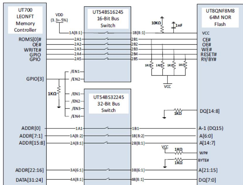
Figure 1. Example Bus Switch \ NOR Flash Configuration
