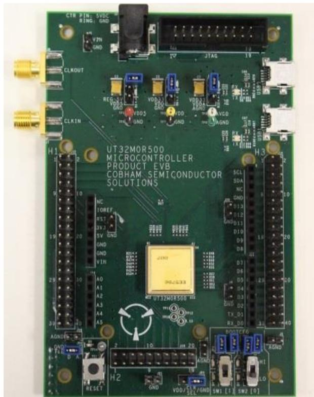
Figure 2: UT32M0R500 Evaluation Board
